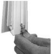
Fasten the profiles together by sliding the square headed bolts into the channel of the profile and attach to the hole in the corresponding bar. Do not tighten the nuts completely until the completed frame is square. **NOTE THAT ALL CONNECTING PROFILES MUST BE FLUSH AND TIGHT TOGETHER TO ENSURE THAT LEAKING IS KEPT TO A MINIMUM.**
